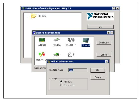
Figure 2-2. Add the Ethernet Interface
