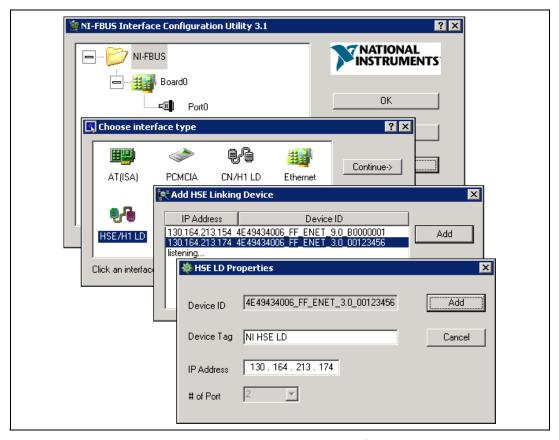
Figure 2-3. Add the HSE Linking Device
