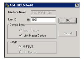
Figure 2-4. HSE Linking Device Port Properties
