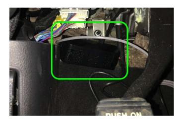
**NOTE:** For the driver's safety, please ensure the DC/DC converter box or wires do not get in the way of vehicle brake or accelerator control.
