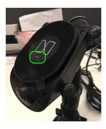
**NOTE:** It may take one minute or more after attaching the device to the power source before you hear the chime. You will also need to view the Nauto device from outside the windshield to see this green light.
