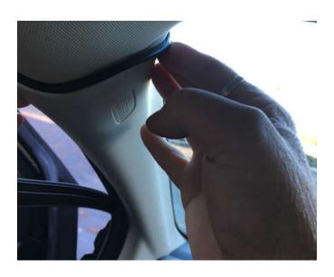
**Step 6:** Run the wires down the A-pillar frame. Making sure the wire always stays on the interior side of the A pillar. Once the wire is set, reattach the rubber door seal.
