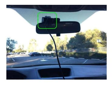
**Step 4:** For a visually clean installation, you can tuck the Nauto wire into the front edge of the headliner, the space between the vehicle windshield and frame.
