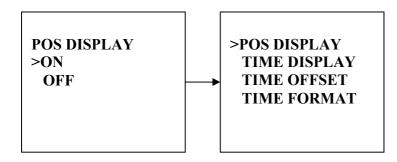
TIME DISPLAY to turn on / off the time display at normal mode
