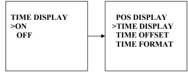
TIME OFFSET to set the add/subtract value from UTC time to equal to local time. When offset value is added, the time will be displayed as LOC instead of UTC
