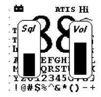
Press volume up/ down to adjust the volume level. A volume sub-menu will appear when press. And timeout after 5 sec.
