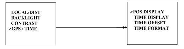
TIME DISPLAY TIME OFFSET TIME FORMAT > COG / SOG POSITION DISPLAY to determine the position data displayed on the normal mode or not
