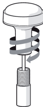
Figure 7 GPS antenna mounting
