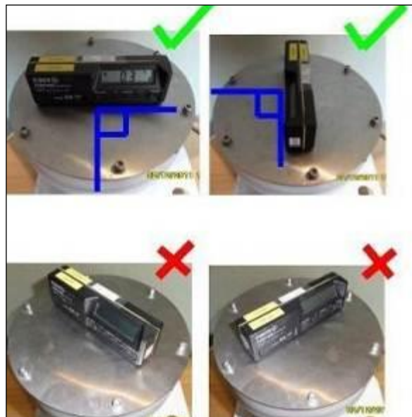
Figure 16 Digital Inclinometer mounted on radar sensor
