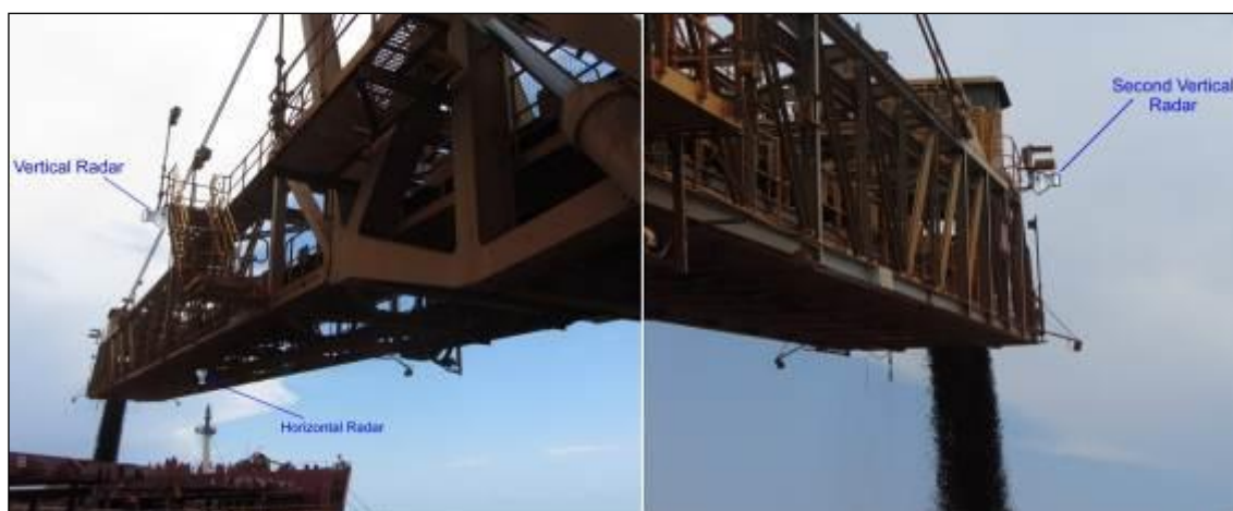
Figure 6 This loader is shown with combined horizontal and vertical scanning radar
