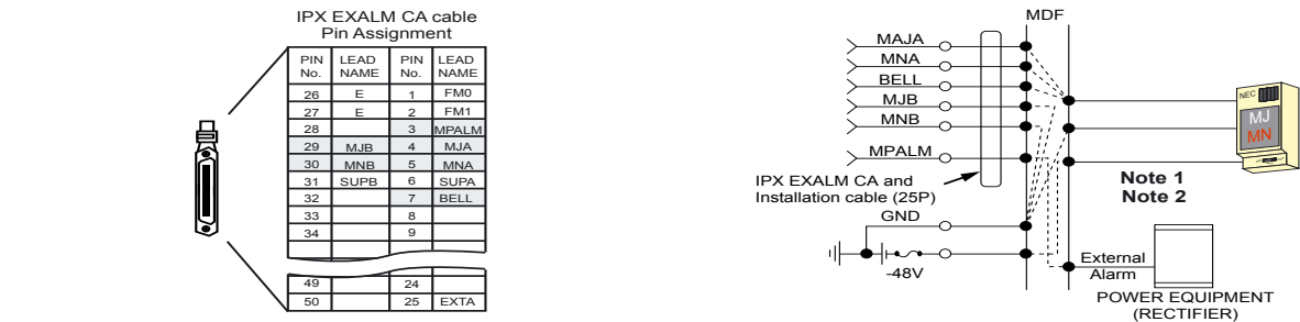
Figure 015-7 Connection of Alarm Indicating Panel (Multiple IMG Configuration)
