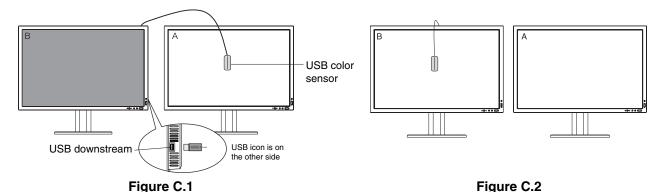
**Display A** – SOURCE display of white point to copy. **Display B** – PA322UHD which performs a copy.
