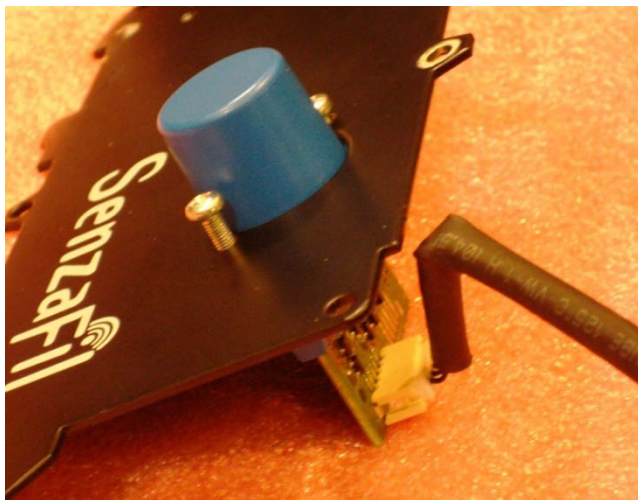
Figure 2d: Luxon Wireless 2450 mechanically secured to the front plate by screws
