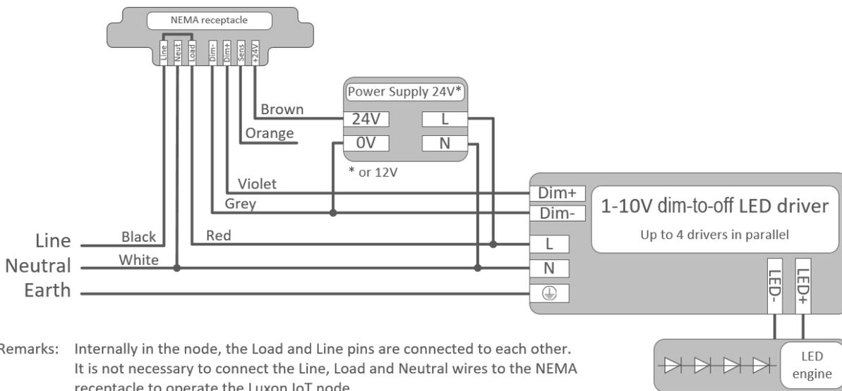
Wiring diagram 3: 1-10V dim-to-off application with Luxon IoT Node Outdoor
