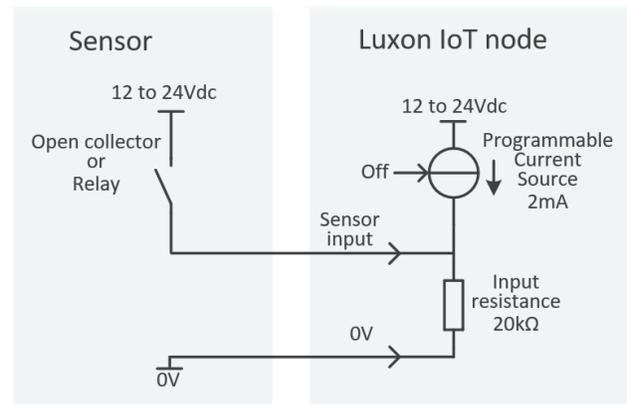
Figure 2: Sensor output switching to 12 to 24Vdc
