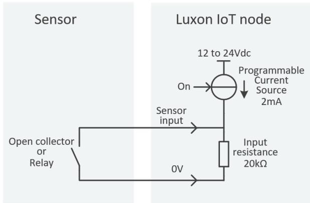
Figure 1: Sensor output switching to 0V.
