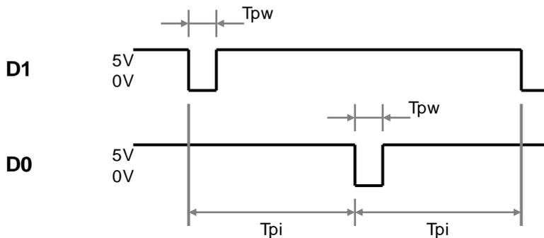
Figure 5: Wiegand protocol timing
