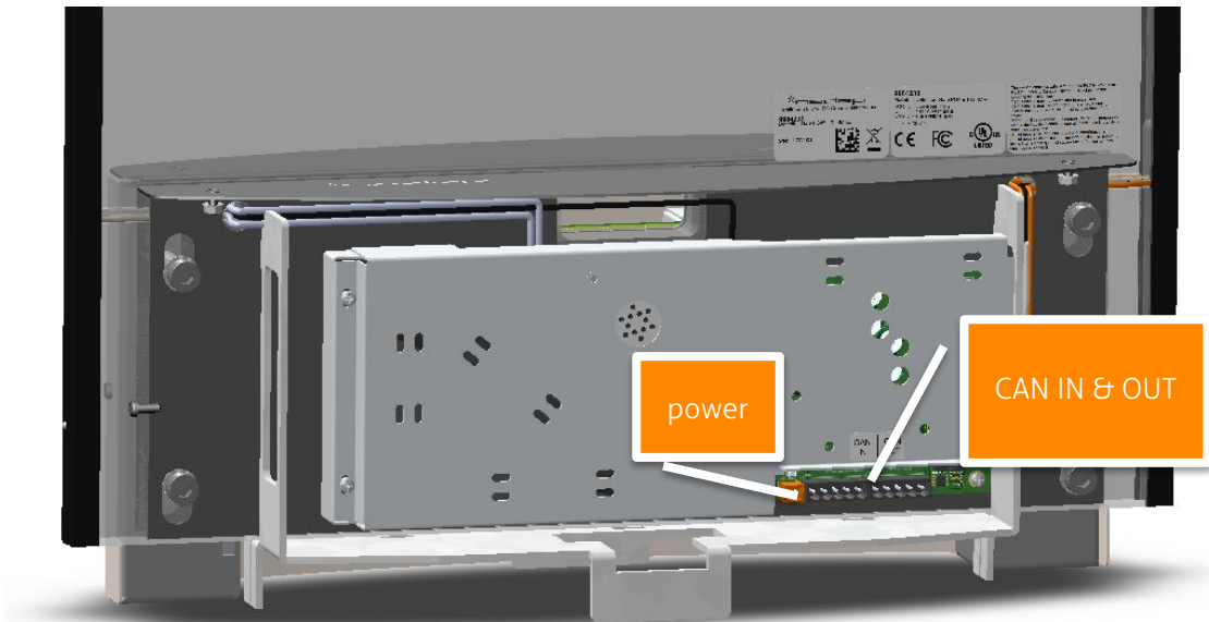
Figure 19 - PG45i match PCB location
