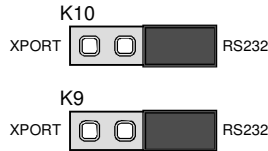
Figure 6: Jumper settings RS232
