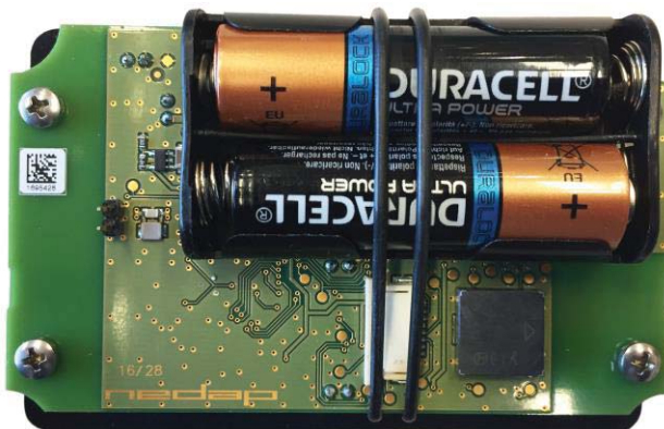
Figure 19: Configuration tool: Battery replacement
