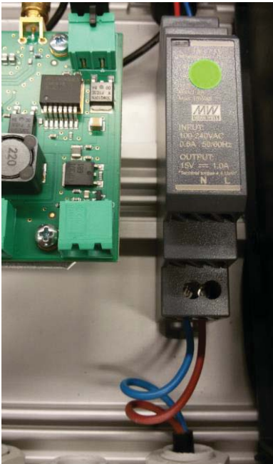
Figure 21: Power supply connection
