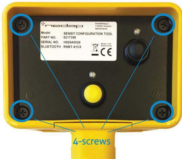
Figure 18: Configuration tool remove screws to open housing
