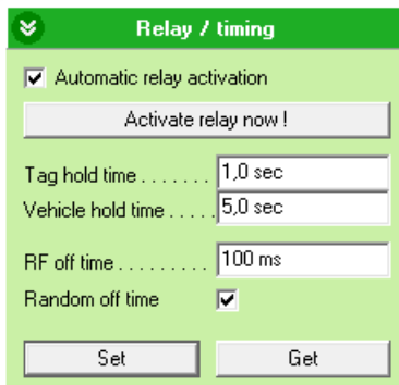
Figure 25: Relay / timing settings
