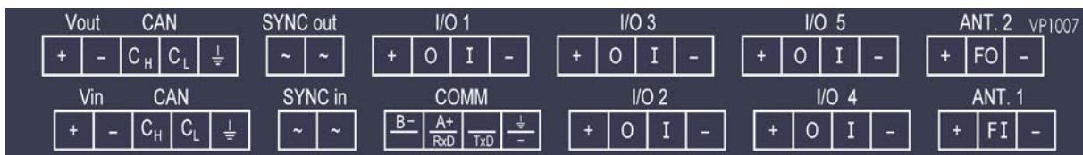
Figure : Sticker on the VP1007 with indication of the connections
