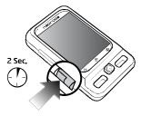
$Press\ the\ on/off\ button\ for\ about\ two\ seconds.\ Release\ the\ button\ when\ the\ device\ starts\ to\ boot\ up.$
