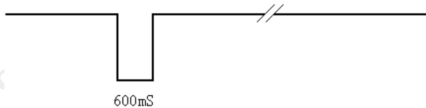
Figure 15 RING Indicator for SMS
