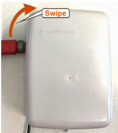
Figure 32 – Magnet Swipe the L900 MIU
