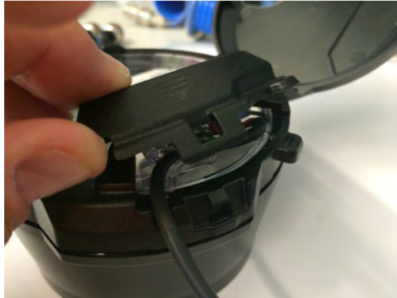
Figure 9 – Covering the Terminal Screws
