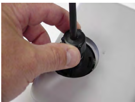
Figure 21 – Gasket and Connector
