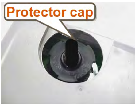
Figure 17 – Black Thread Guard from Male F-Connector
