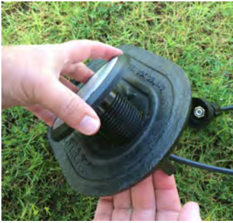
Figure 13 – Inserting the Antenna into the Pit Lid
