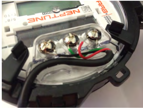
Figure 7 – Cable Threaded Around Strain Relief Posts
