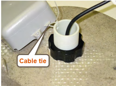
Figure 31 – L900 MIU Attached to Antenna
