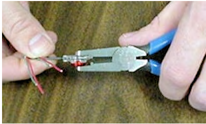
Figure 25 – UR Crimping Tool
