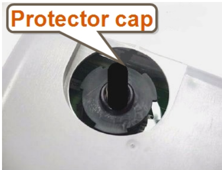
Figure 30 – Black Thread Guard from Male F-Connector
