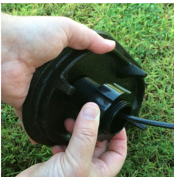
Figure 28 – Securing the Locking Nut
