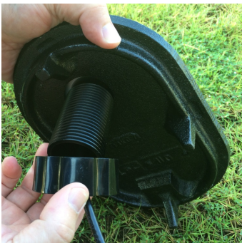
Figure 27 – Locking Nut on Antenna
