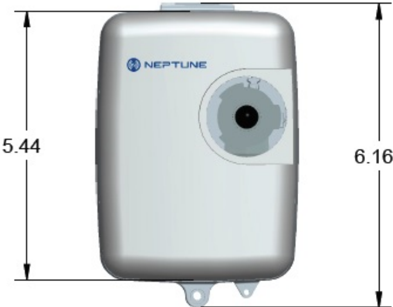
Figure 3 – L900 MIU - Pit Dimensions - Front
