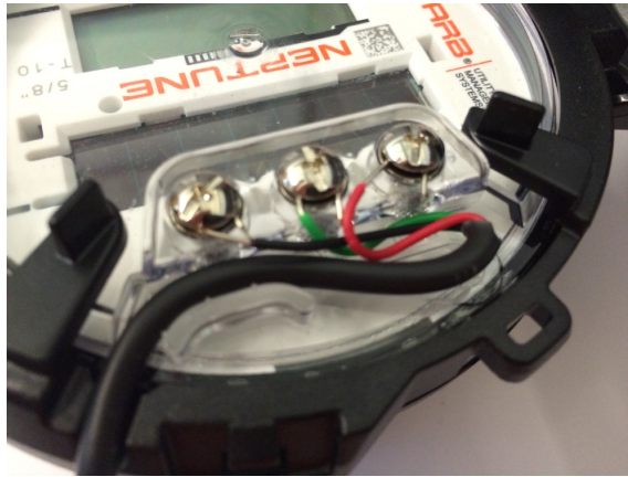
Figure 10 – Cable Threaded Around Strain Relief Posts
