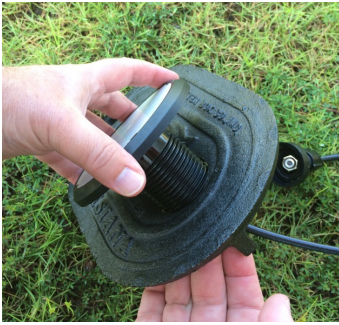
Figure 26 – Inserting the Antenna into the Pit Lid
