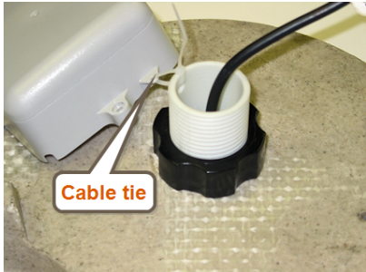
Figure 44 – L900 MIU Attached to Antenna
