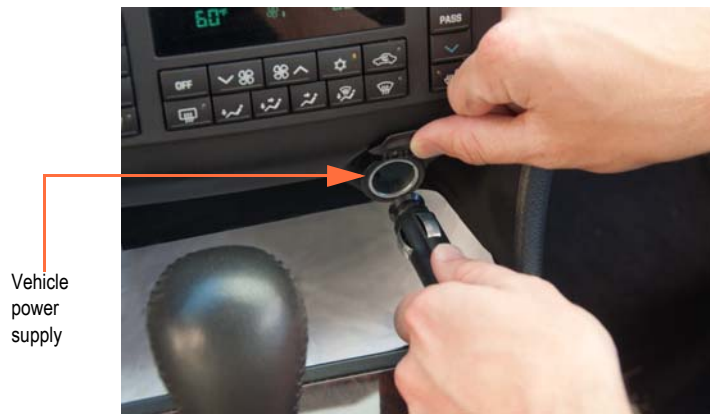
Figure 3.26 Vehicle Power Supply Cable Inserted In Car
