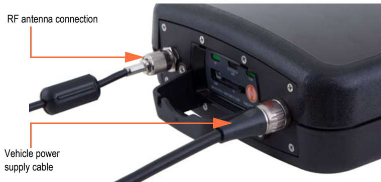
Figure 3.25 Vehicle Power Supply Power Cable
