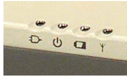
Figure B.9 LED Power Indicators
