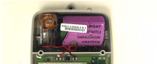
Figure 44 Returning Spliced Battery to Main Housing
