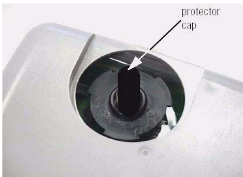
Figure 14 Black Thread Guard from Male F-Connector
