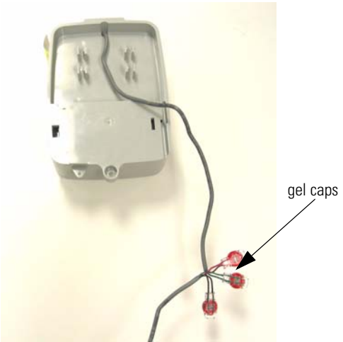
Figure 33 Gel Cap Connections
