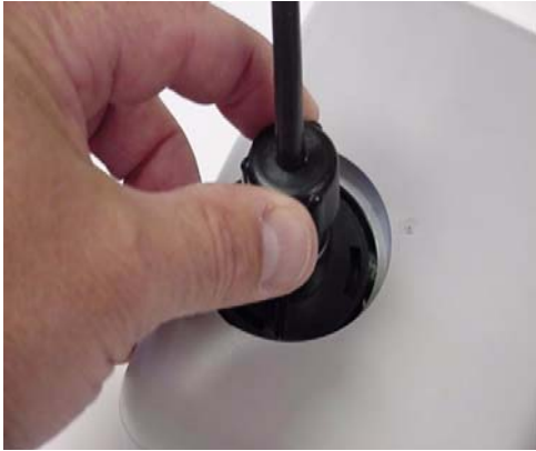
Figure 18 Black Cone-Shaped Gasket and Connector
