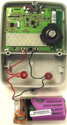
Figure 42 Splicing the New Battery
