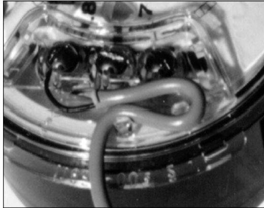
Figure 6 Cable Threaded Around Strain Relief Posts
