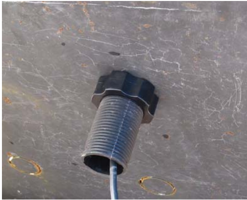
Figure 13 Locking Nut on Antenna
