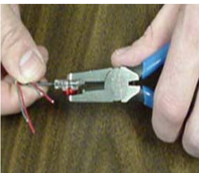
Figure 23 UR Crimping Tool
