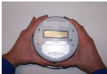
Figure 7 – Removal of Electronics Housing
