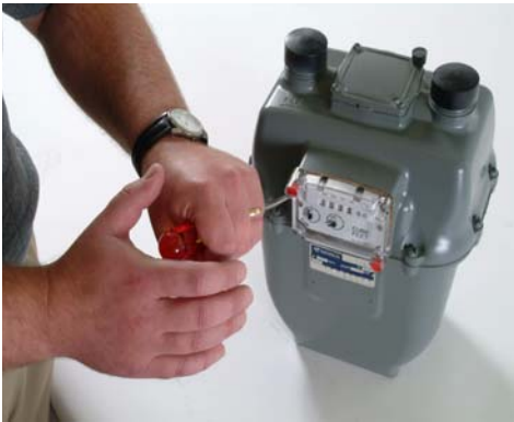
Figure 13 Puncturing and Removing Tamper Plugs
