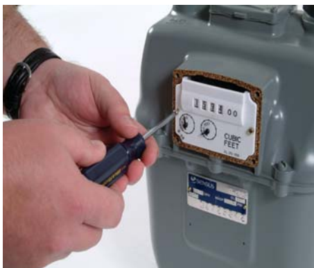
Figure 15 Removing Index Mounting Screws
