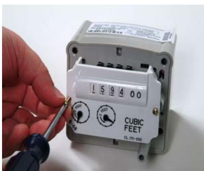
Figure 17 Securing the Index
