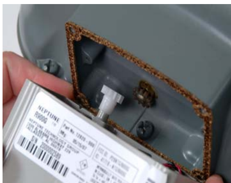
Figure 18 Mount the R900G
