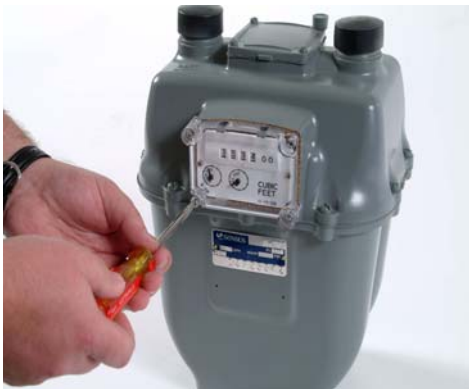
Figure 14 Removing Lens Mounting Screws
