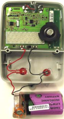
Figure 12 Splicing the New Battery
