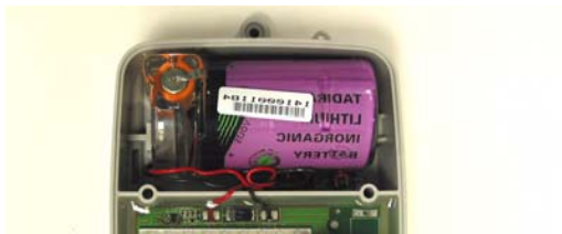
Figure 14 Returning Spliced Battery to Main Housing
