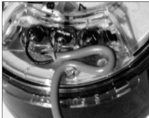
Figure 6 Cable Threaded Around Strain Relief Posts
