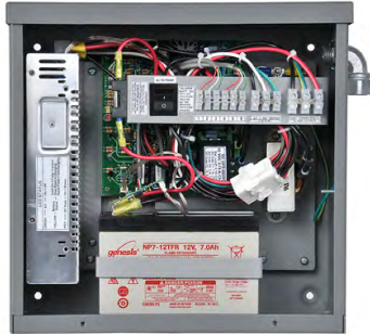
Figure 39 – Wire Input and Output Connectors
