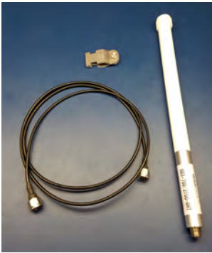
Figure 10 – Items for Cellular Antenna
