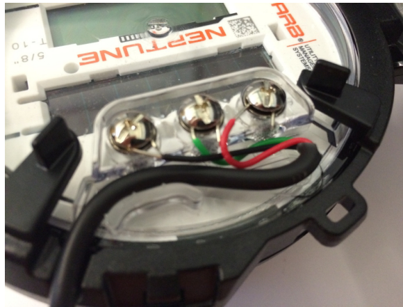
Figure 10 Cable Threaded Around Strain Relief Posts
