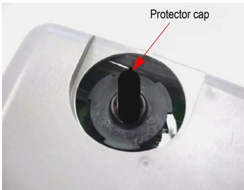
Figure 30 Black Thread Guard from Male F-Connector
