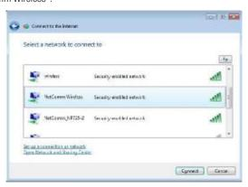
4. Tick "Display Characters" and type in the network security key. This example uses "a1b2c3d4e5". Then click "Connect".
