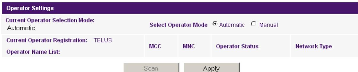
Figure 28 - Advanced View – Operator Selection
