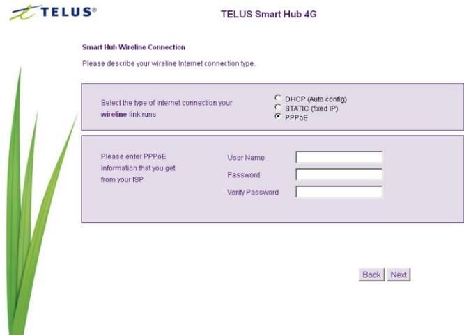
Figure 11 - Startup wizard - AssureNet Service Settings - Connection Type - PPPoE
