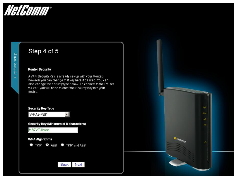
Figure 6 - Startup Wizard - Wi-Fi Security Settings
