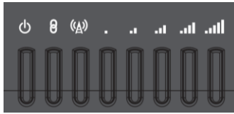
Figure 2 - NTC-140-01 router LED Indicators
