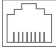
Figure 129 -The RJ-45 connector
