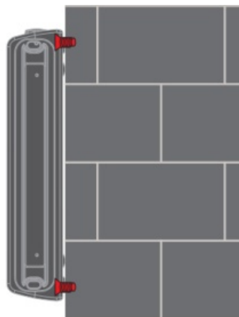
Figure 4 - Wall mount - Flat against the wall
