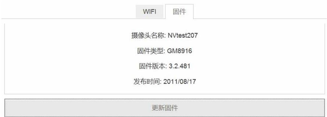
On the firmware page, information includes camera name, firmware type, firmware version, and release date. Click **Update firmware** to complete. There will be prompt to restart the camera.
