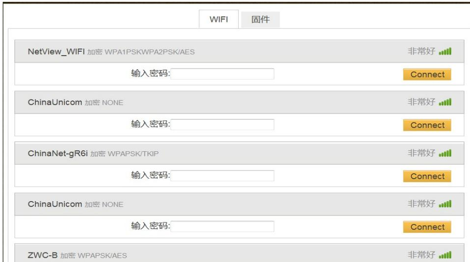
If the below prompt appears, it means that the wifi is being configured. User can close this window after several seconds. Then remove the network cable and repower the camera.
