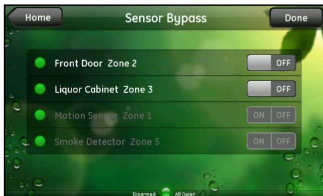
Figure 13. Choose sensors to temporarily bypass
