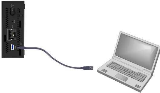
Figure 4. Connecting the WNCE3001 to a laptop
