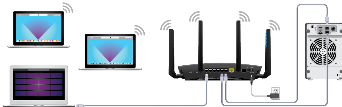
Figure 5. Ethernet port aggregation
