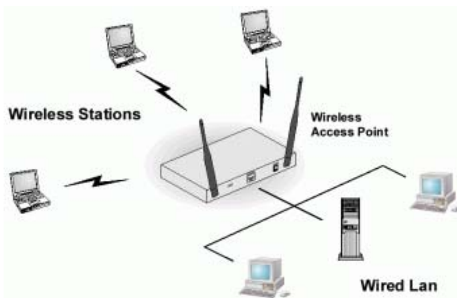
Figure 1: Wireless Access Point
