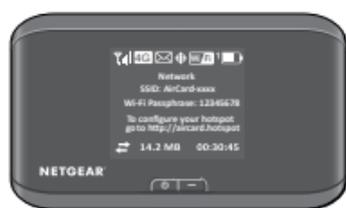
**Note:** The LCD screen goes into sleep mode to save power. To wake up the LCD screen, **press** and **release** the Power key.
