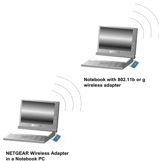
Figure 5-2: NETGEAR MA701 Wireless PC Card in Peer-to-Peer Mode
