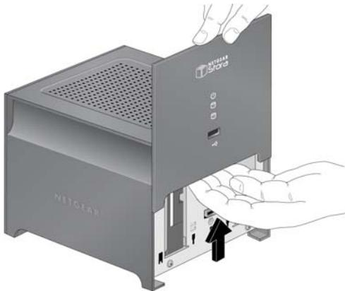
3. Press the lever on the back of the unit to unlock the drive.
