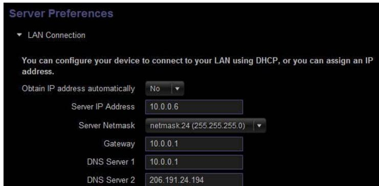
The Obtain IP address automatically drop-down menu controls whether Stora obtains a dynamic IP address from the router.
