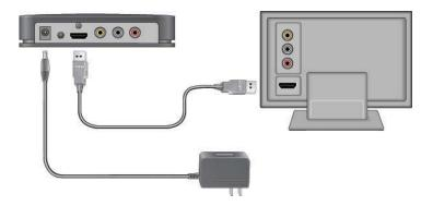
The Push2TV adapter LED is red when the adapter powers up. Then the LED turns amber to indicate the adapter is ready, but is not yet connected to your computer.
