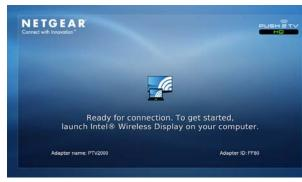
If you do not see this screen, make sure the TV input is set to the port where the Push2TV adapter is connected and all cable connections are firmly secured.
