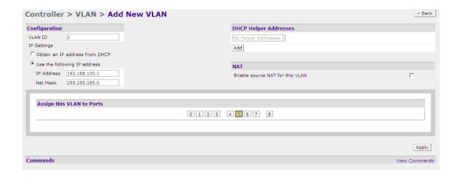
The example shows how to create VLAN 100 and configure Port 0/6 and 0/7 to be part of the VLAN.
