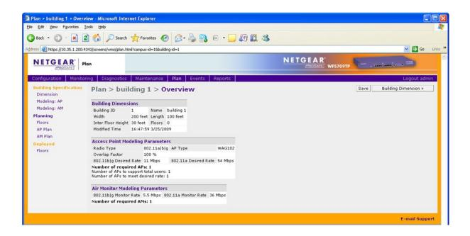
3. On this screen, select "Unit" as Feet or Metres, and fill in the rest of the details. In this example, the RF plan is only for the top floor of a 2-floor building, so "Floors" =1. Note that the dimensions are for the full area covered by the floorplan .jpg that will be loaded at a later step, which may be slightly larger than the area covered by the physical building. Click "Apply", then "AP Modelling Spec".
