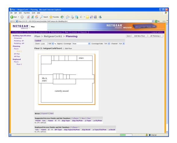
10. If there are any areas on the floorplan where coverage is not required or is optional, click "New" in the "Areas" menu. In the Area Editor, specify coordinates to indicate the area where coverage is not required, select "Don't Deploy" or "Don't Care", and click "Apply".
