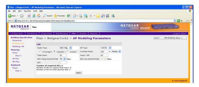
6. The Air Monitor Modelling Parameter screen determines how many AMs will be required. In most cases, default settings will be suitable. Click "Apply", the "Save", then "Planning".
