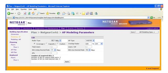
5. Edit the default AP parameters as required. "Coverage" will calculate required number and location of APs based on the area to be covered, while "Capacity" will calculate this based on number of users to be supported. 100% Overlap Factor indicates that the AP coverage areas should just touch, increasing this parameter will make roaming more reliable. The parameters specified on this screen will determine how many APs are required. Click "Apply", then "AM Modelling Spec.".
