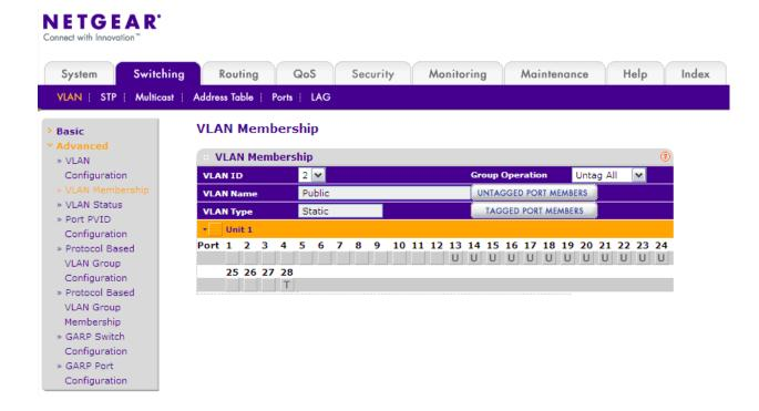
Configure PVID settings – ports 1 to 12 with PVID of 1, ports 13 to 24 with PVID of 2. PVID on trunk port (port 28) is not relevant.
