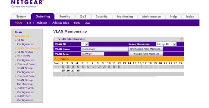
Add ports 13 to 24 untagged to VLAN2. Add port 28 tagged to VLAN2.
