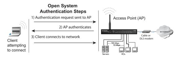
Figure 6-1: Open system authentication
