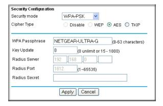
Figure 4-9: WPA-PSK Security Configuration
