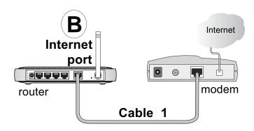
Figure 3-2: Connect the wireless router to the modem
