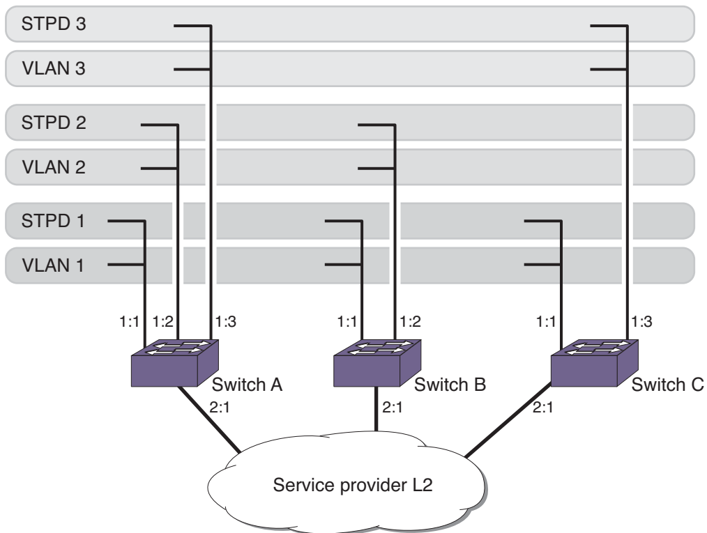
Figure 34. Sample Network Using STPD BPDUs Tunneling
