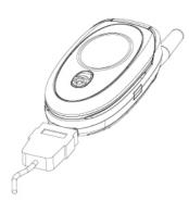
Your phone is powered by a rechargeable battery. A new battery must be charged for 2 hours at least before being used for the first time. It reaches its optimum capacity after a few cycles of use.
