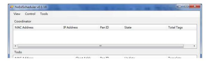
A: If MAC address does not show up normally, insert a paper clip or a SIM-eject tool to the reset hole of coordinator, press and hold the reset button for 2 seconds to reset the coordinator.
