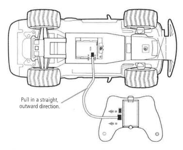
Remove and discard the demo wire which runs from the vehicle to the controller.
